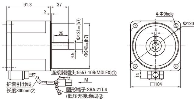
①Connector: 5557-10R (MOLEX) ②Lead wire length 300mm ③Round terminal: SRA-21T-4 (low ground)
