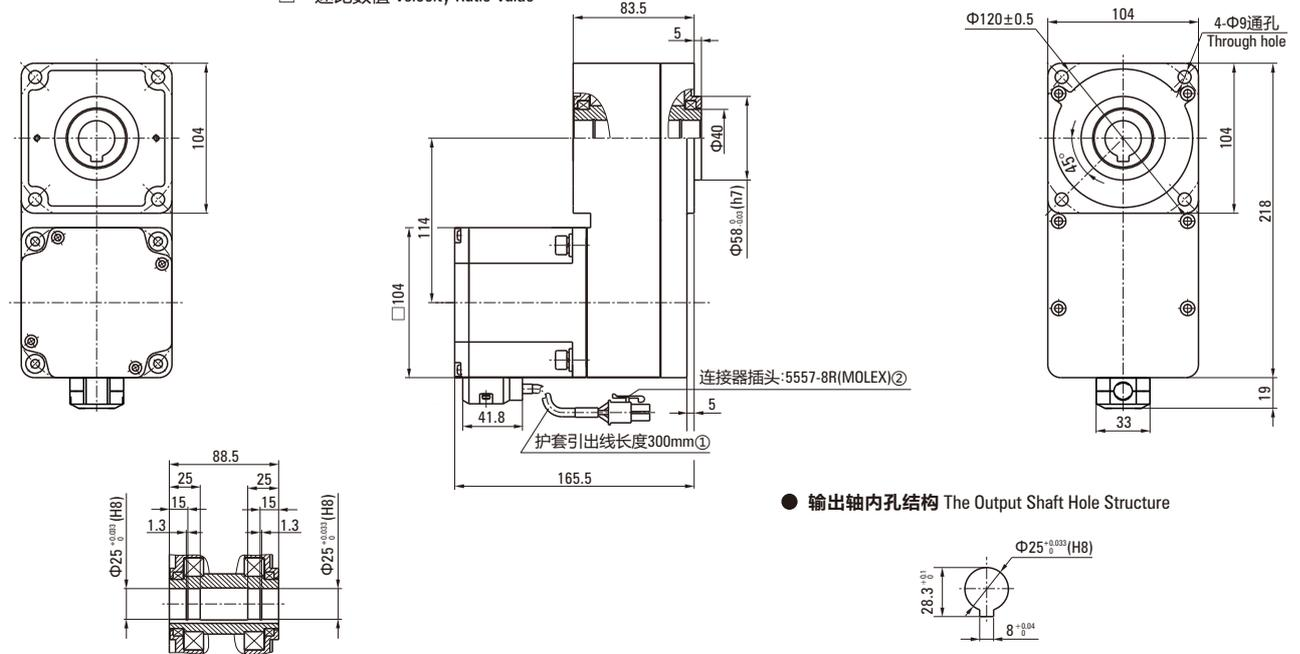
● 输出轴内孔结构 The Output Shaft Hole Structure
